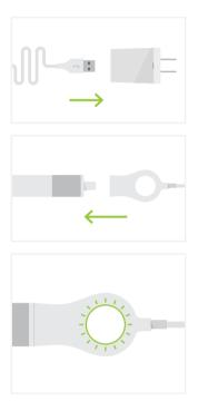
Plug the USB connector end of the charging connector into the USB wall adapter.
