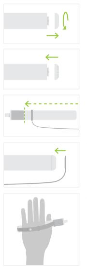
Swivel the end cap counter-clockwise to unlock and pull to remove.
