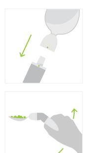
Connect the attachment to the handle using the gray dots for correct alignment. It will snap in place using magnets.
